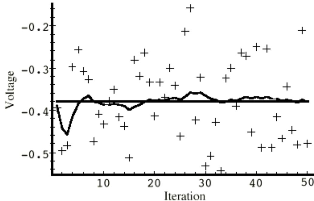
**Figure 3-1.** The first simulation:  $R = (0.1)^2 = 0.01$ . The true value of the random constant  $x = -0.37727$  is given by the solid line, the noisy measurements by the cross marks, and the filter estimate by the remaining curve.
