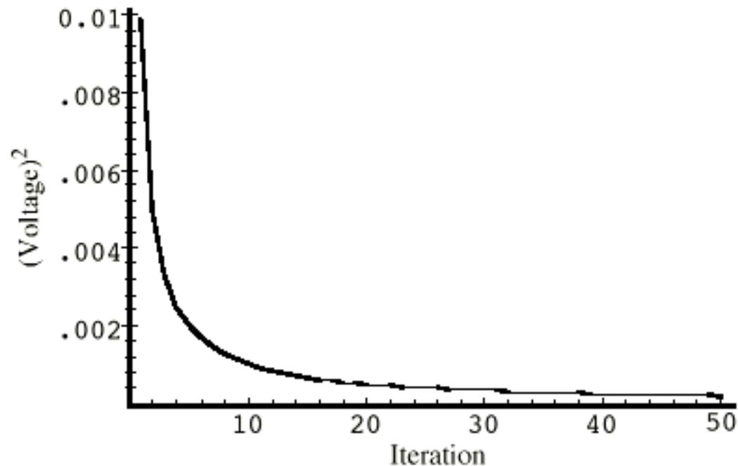
**Figure 3-2.** After 50 iterations, our initial (rough) error covariance  $P_k^-$  choice of 1 has settled to about 0.0002 (Volts<sup>2</sup>).
